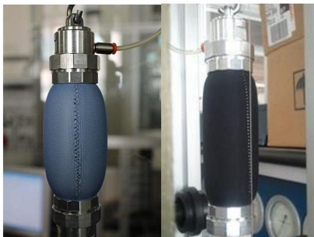
**Figure 2.** Prototypes of textile pneumatic muscles of Politecnico di Torino: (a) warp and weft fabric; (b) knitting fabric.
