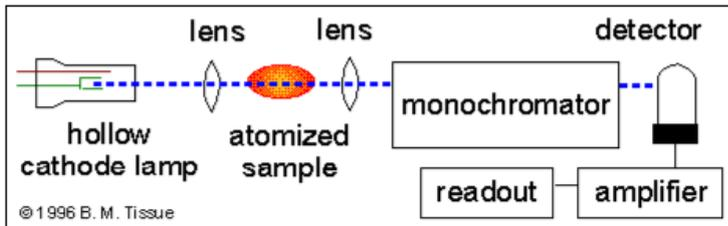
This is universally accepted technique, most of the researcher working on this technique. Absorption is so sensitive that it can measure down to parts per billion of a gram ( $\mu\text{gdm}^{-3}$ ) in a sample. The technique makes use of the
