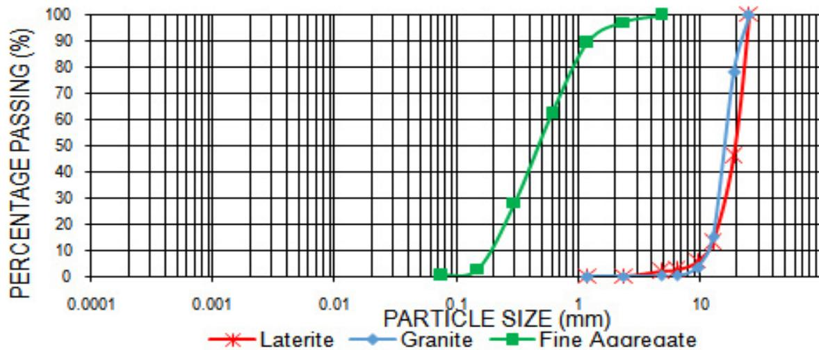
**Figure 3.** Particle size curves of lateritic nodules <sup>[6]</sup>.
