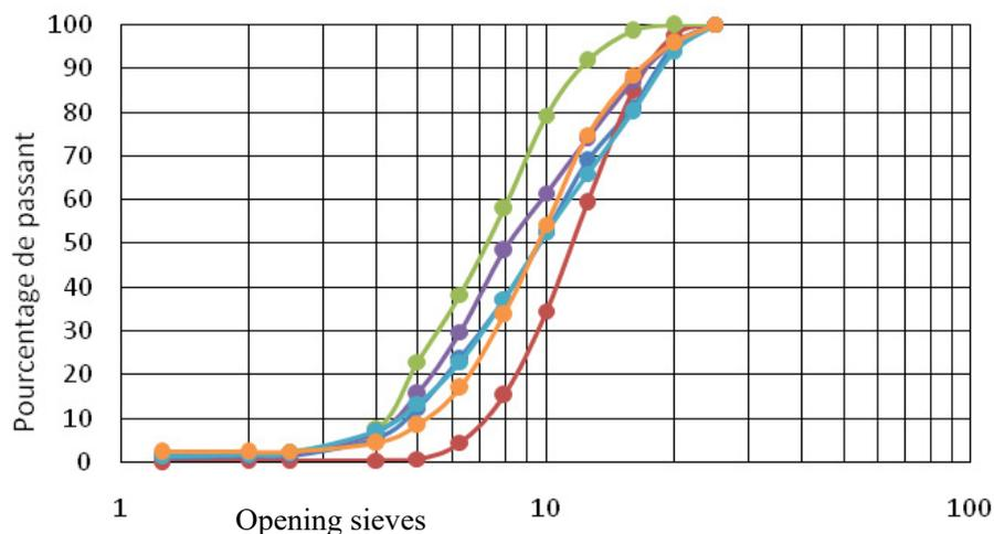
**Figure 4.** Particle size curves of lateritic nodules <sup>[11]</sup>.
