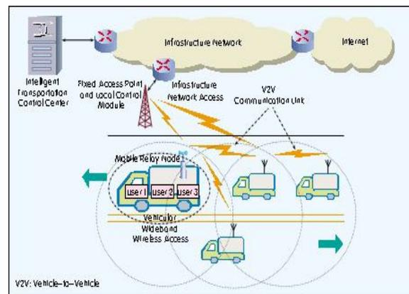
▲ Figure 2. The proposed heterogeneous vehicular communication architecture.
