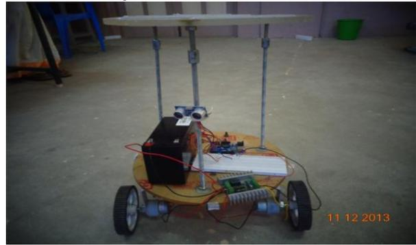
Fig. 7 Object detection and avoidance by using Ultrasonic sensor
