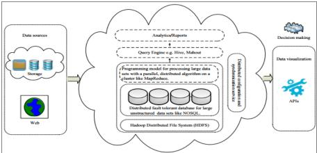
Fig. 1. Diagram showing cloud computing usage in big data.
