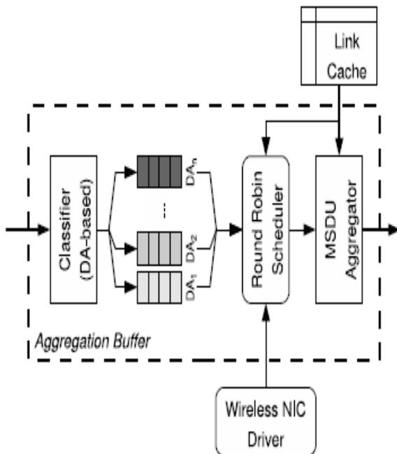
Figure. 1. Block diagram for the packet aggregator
