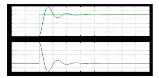
Fig 4.Simulation response of Phase and Gain Margin without Fuzzy controller.
