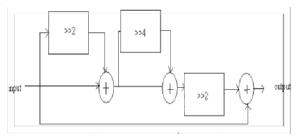
Figure 7. Block diagram of bit parallel multiplication by  $1/\sqrt{2}$
