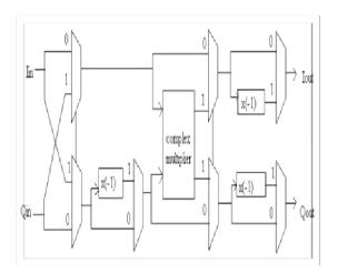
Figure 9. Block diagram of complex constant multiplier
