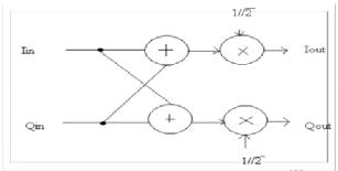
Figure 8.Block diagram for multiplication by  $W_N^{\ N/8}$
