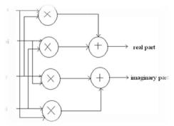
Figure 6. Block Diagram Of Conventional Complex Multiplier Structure
