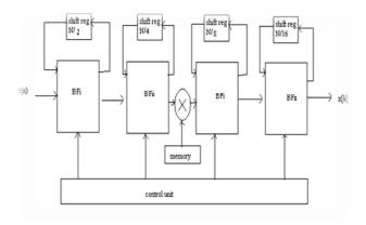
Figure 5. Block diagram for pipelined FFT
