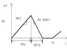
Fig.3 DCM Inductor Current
