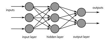
Fig. 5 Model of a Typical Multilayer Artificial Neural Network
