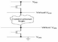
**Fig1: Basic Power Gating Circuit**
