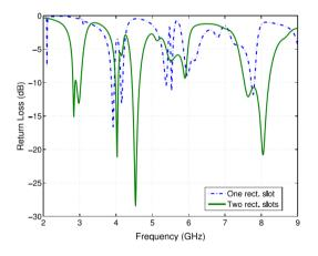
Figure 3: Effect of return loss of the proposed antenna due to the slots on the patch.
