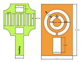
Figure 1: Configuration of the proposed antenna.
