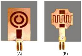
Figure 2: A fabricated proposed antenna used in the experimental setup (A) Bottom view (B) Top view of antenna.
