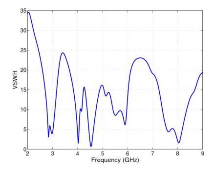
Figure 5: VSWR of proposed antenna design.
