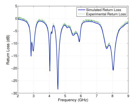
Figure 4: Simulated and measured (experimental) results of return loss of the proposed antenna design.
