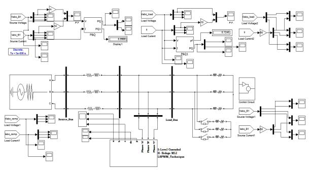
Fig.6.Closed loop simulation circuit of shunt active power filter
