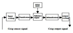
Fig.1. Block diagram of a fuzzy logic controller.
