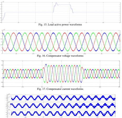
Fig.18. Three Phase Multi Level Inverter Output Voltage
