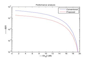
Figure 3: BER performance comparison for Conventional OFDM system versus Conventional OFDM system.
