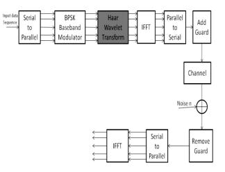
Figure 1: The proposed Haar wavelet based BPSK OFDM system.
