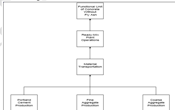
Figure II-2 Production of Concrete
