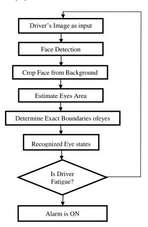
Figure: 1. Flow chart for fatigue detection system
