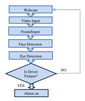
Figure 2: Flowchart of Driver Drowsiness Detection System
