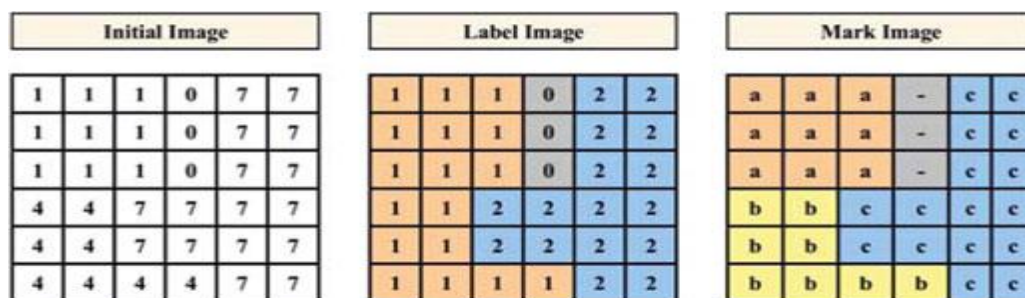
Fig. 4. Automatic identification of objects using L-shaped masks (3 Objects a, b, and c are identified).
