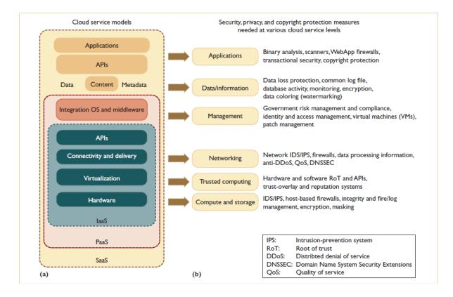
Figure 1. Three cloud service models. (a) Infrastructure as a service (IaaS) is built on top of virtualized compute, storage, and network resources, platform as a service (PaaS) at the OS/middleware level, and software as a service (SaaS) at the user application level. Each service level requires (b) different security, privacy, and copyright protection measures.
