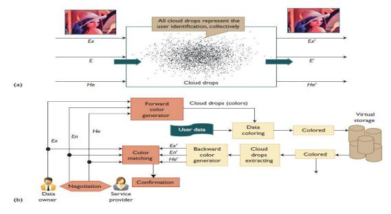
Figure 4. Data coloring This coloring method enables trust management at various security clearance levels in an open data center. We can see (a) forward and backward data coloring processes by adding or removing unique cloud drops (colors) in data objects. We also demonstrate (b) data coloring and user identification color matching through trust negotiation.
