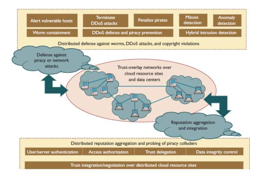
Figure 3. Distributed-hash-table (DHT)-based trust-overlay networks. We build these networks over cloud resources provisioned from multiple data centers for trust management and distributed security enforcement.
