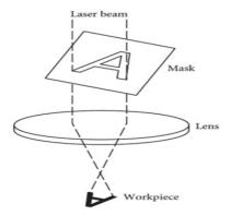
Figure 1: Mask engraving technology.
