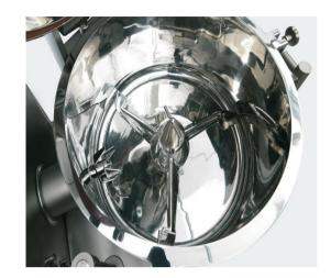
Figure 1: High shear granulator mixing bowl with impeller and chopper blades.
