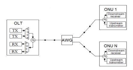
Fig.4. WDM-PON architecture
