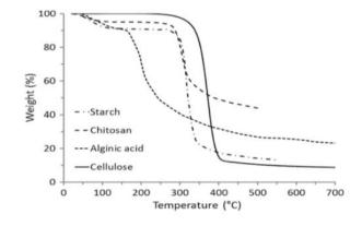
Figure 2. Thermogravimetric curves of selected carbohydrate flame retardants <sup>[11]</sup>.
