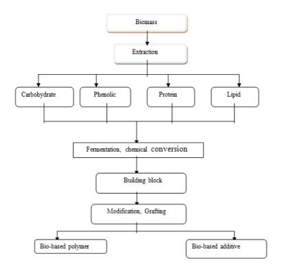
Figure 1. The process of obtaining bio-based additives for polymer <sup>[4]</sup>.
