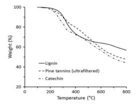
Figure 3. Thermogravimetric curves of selected Phenolic Flame retardant compounds <sup>[8,17]</sup>.
