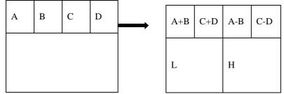
Figure1: The horizontal operation on first row
