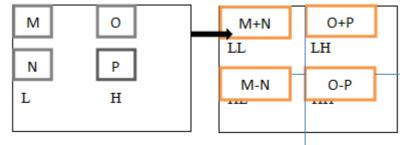
Figure 2: The vertical operation
