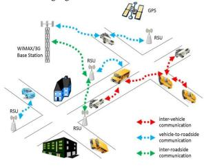
Fig 1.Simple Representation of RSU in VANET
