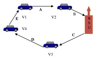
Fig 2. Sending a packet from a vehicle to an RSU
