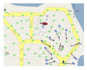
Fig.3.Example of an RSU choosing a road to send a packet to
