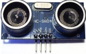
Figure 7- Pin Diagram of Ultrasonic sensor
