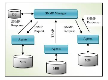
Fig 1. Centralized NMS architecture
