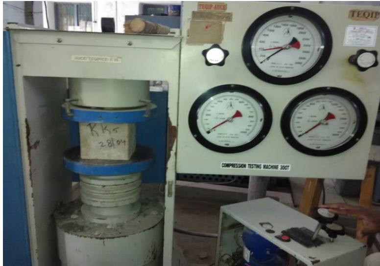
Fig 1. Testing of cubes in Compression testing machine
