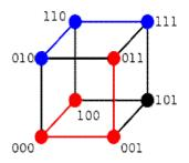
Red path has a hamming distance of 3(100 requires all 3 bits changed to get to 011) Blue path has a hamming distance of 2(010 requires all 2 bits changed to get to 111).
