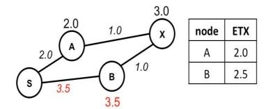
Fig.2. An example of a routing outley inconsistency in PPS without relaxing the loop-detection condition.
