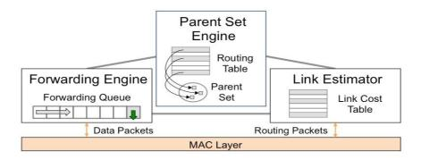
Fig.1. Main components of CTP+PPS.
