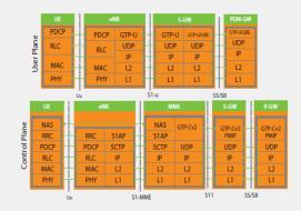
Figure 6: LTE User-Plane and Control-Plane Protocol Stacks
