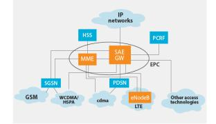
Figure 3: Simplified View of LTE Network Architecture
