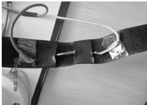
Photograph of seat belt sensor (Reed switch) provision
