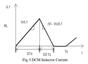
D2 or D3 in DCM operation becomes an additional unknown in addition to D. This division of the D' intervalinto D2 and a new D3 interval usually happens when I(out) has a minimum DC value called the critical current, Icritical. DCM usually occurs at light load and Vout jumps up from its CCM value, sepic converter, to a higher value output-voltage. This can be very useful for power supplies employed for starting fluorescent lights, which initially have zero load.
