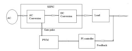
Figure.1 Block Diagram
