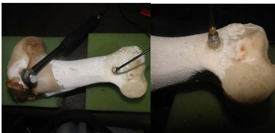
Figure 4. The modal test experiment setup.
