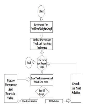
Figure 6: A generic process flow of ACO.
