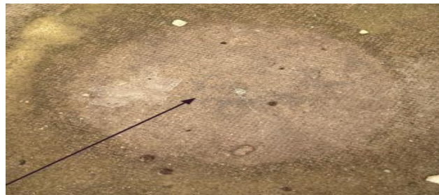
Fig. 6 Shows a mossy tile when sprayed with nano composite(mixed grapheme oxide and titanium dioxide),it removes algae on the surface.
