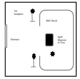
Figure 3. Typical air sampling set-up during a spill condition
