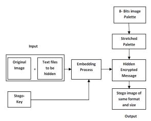
Figure - 1: Sender's View of Steganography Techniques.
