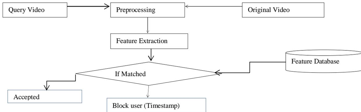
Fig. 1. A framework of video copy detection system.
