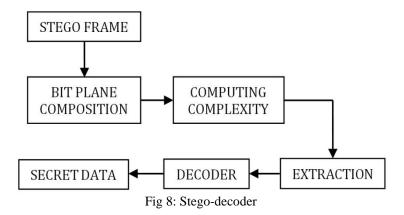
Fig.8.represents the block diagram of stego decoder in which the stego frame is decomposed into bit plane and complexity of each bit plane is calculated and the secret data embedded in frame is extracted.
