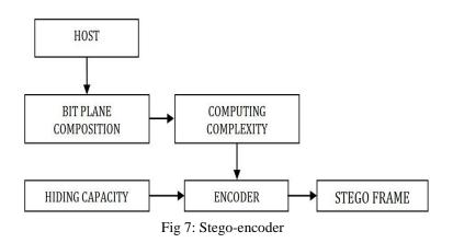
Fig.7. represents the block diagram of stego encoder in which the image frame of video is decomposed into planes and complexity of each plane is calculated using (1). More complexity of frame more data can be embedded in carrier. Thus the frame generated is called as stego frame.
