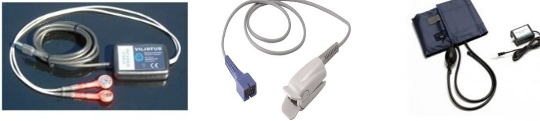
Figure.7 Pictorial view of Pulse Oximeter and BP sensor.
