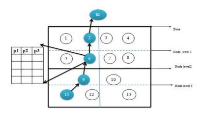
Figure 2.1 Zone based routing in DMP
