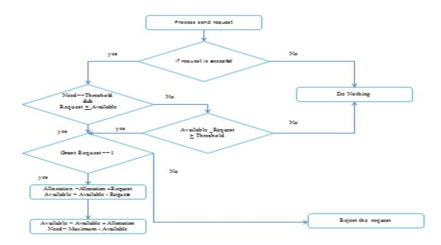
Figure 3.2 Working principle of TRA
