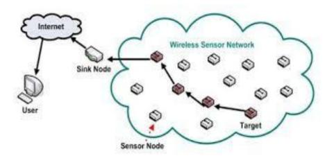
Figure 1.1 Wireless Sensor Network
