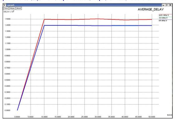
Fig. 2.comparison of Delay between AODV, proposed Genetic Algorithm and LDT
