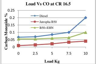
Fig. 5 Variation of CO emission with load of engine for different fuels
