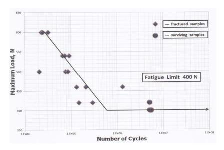
Graph 2. A study of stress fractures using dynamic loading on "Unique" implants with a 3 mm diameter and a 25° angular titanium-abutment.
