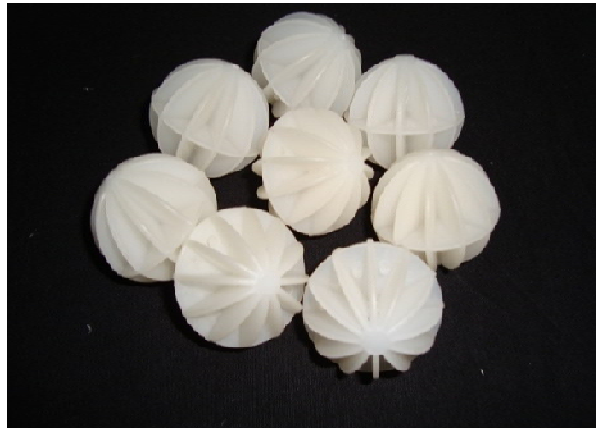
Fig. 2 Photograph of the polypropylene polyhedral spherical balls (Packing media)
