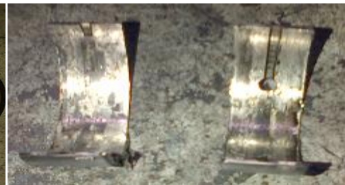
Fig.4. Scratches on upper main bearing caps
