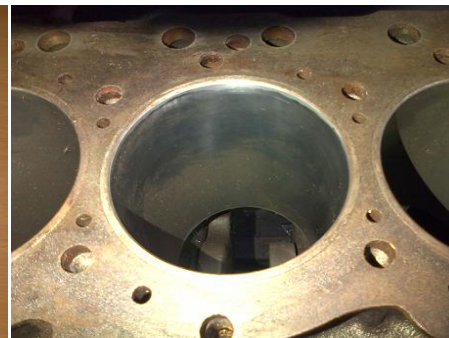
Fig.6. Cylinder in good condition
