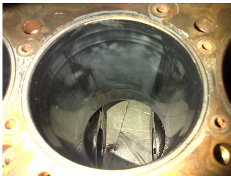
Fig.8. Worn out cylinder surface
