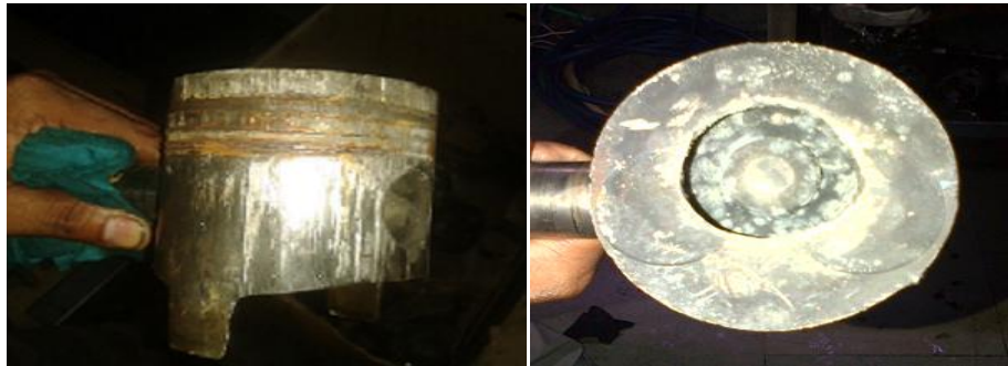
Fig.7. Worn out piston due to overheating
