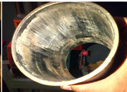
Fig.9. Worn out piston sleeves due to seizing of badly overheated piston
