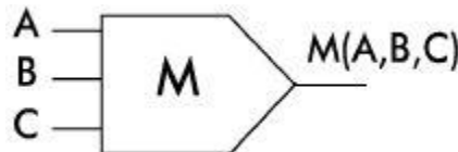
Fig.7. Structure of Majority gate
