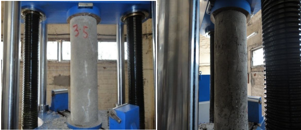
Fig. 1 - Compression test on circular bamboo reinforce concrete column.
