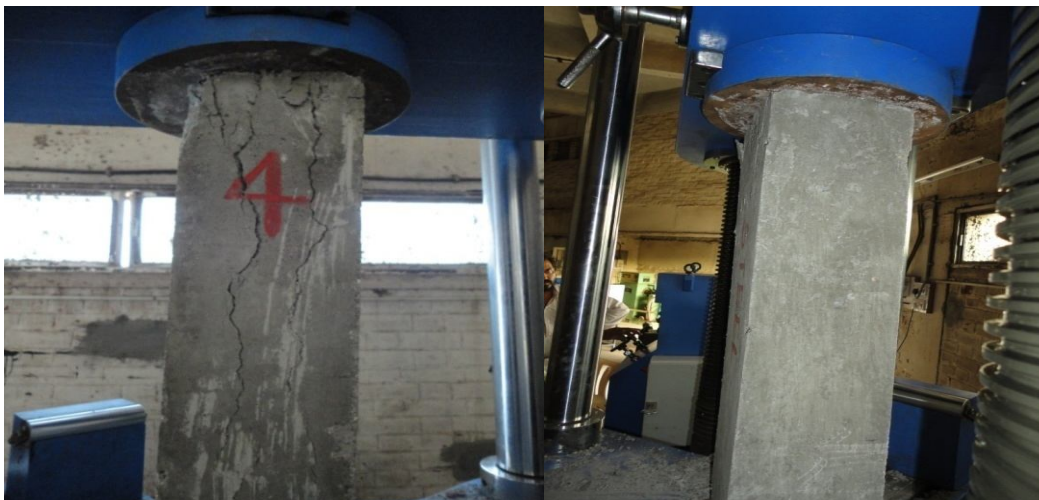
Fig. 3 - Failure of square bamboo reinforce concrete column
