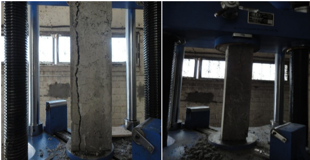
Fig. 2 - Failure of rectangular bamboo reinforce concrete column.
