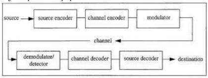
Figure 4 Block Diagram of Digital Communication
