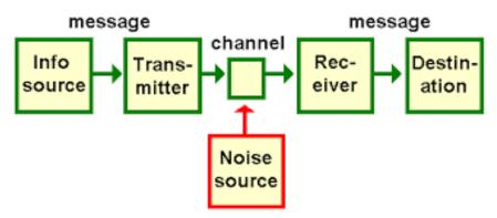
Figure 3 Block Diagram of Analog Communication
